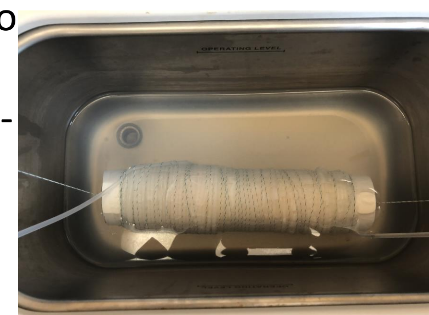
Fig.3 – tubing inside sonicator
