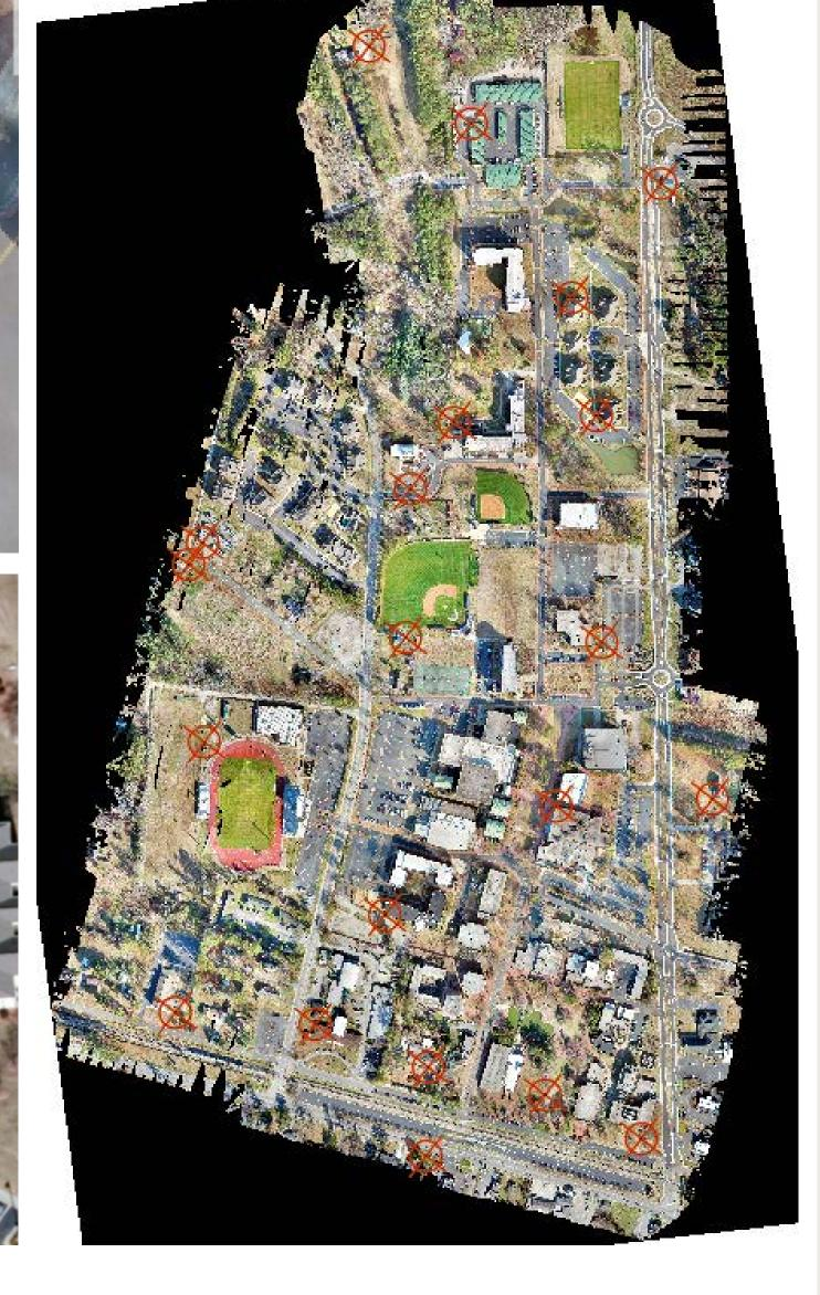
The orthomosaic raster is brought into ArcGIS Pro for a minor transformation to be georeferenced to existing aerial imagery. To align the image I had to add control points to fixed locations after which the transformation was applied.
