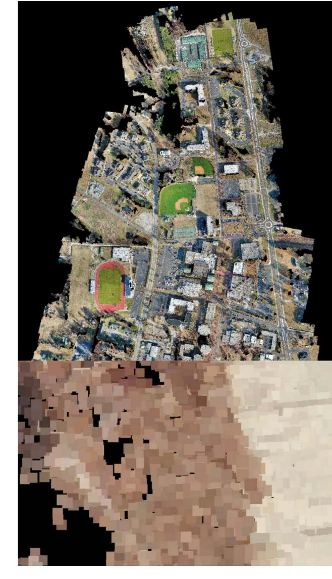
On the left is 1,797 photos taken from a drone after being aligned using the GPS coordinates that were gathered for each photo during the flight. On the right is a georeferenced photo created by the software through mosaicking. The process involved several steps including creating a point cloud by comparing the images, a polygonal mesh is built from the point cloud, the mesh is used to generate a Digital Surface Model (DSM), and the DSM and images are used to generate the Orthomsaic.
