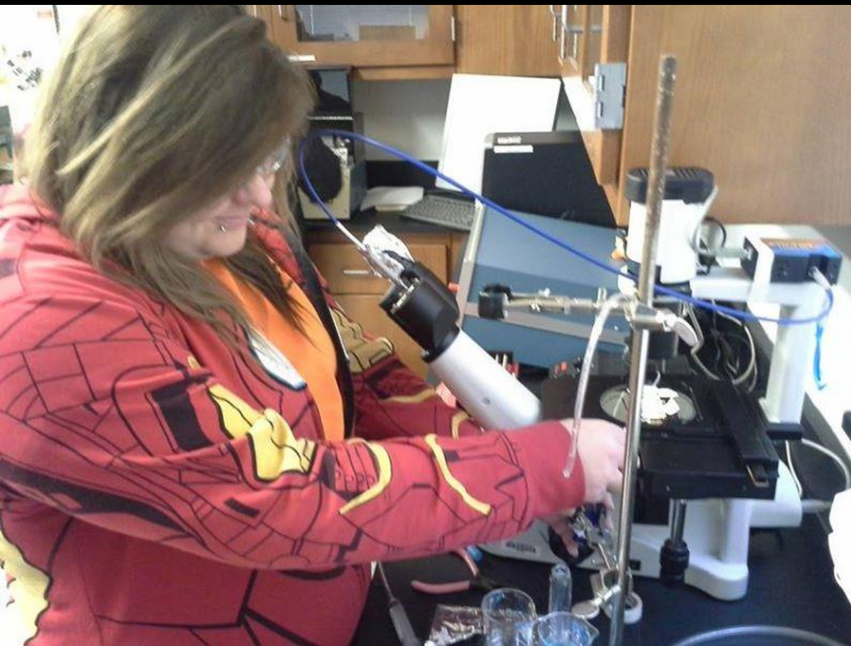
2013: Jessica Stancil preparing for spectral measurements with a microscale flow cell
