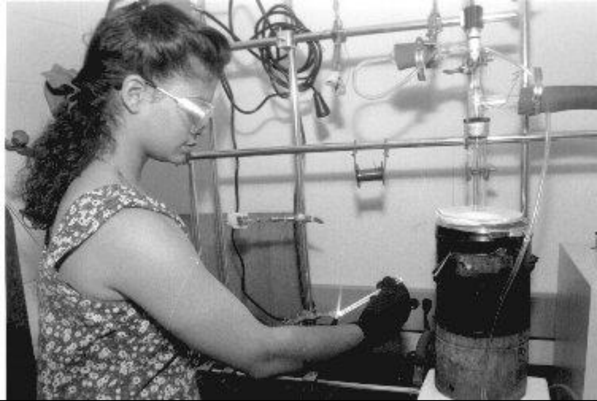
1995: Amy Chavis torch-sealing a glass ampoule.
