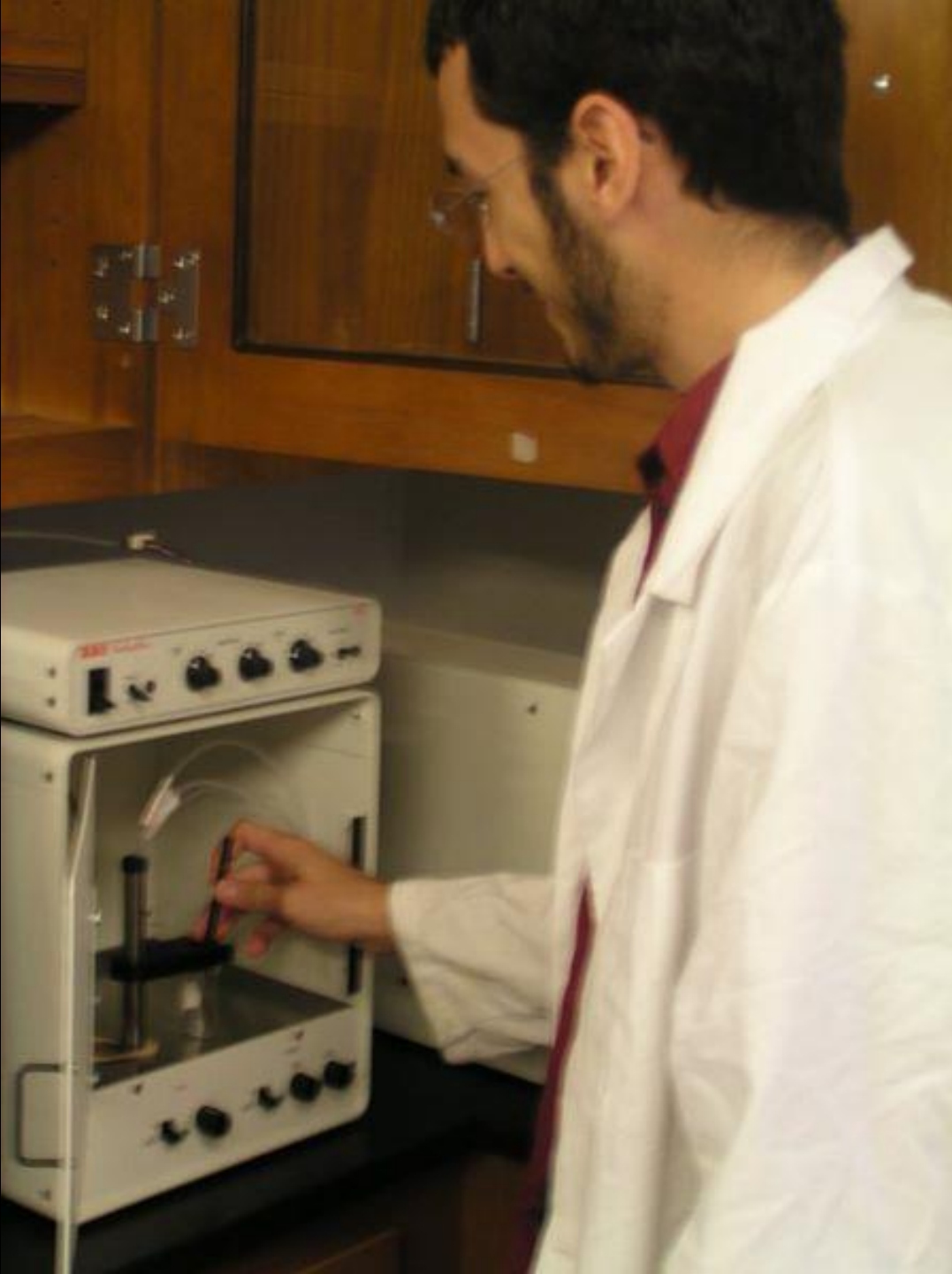
2007: Shane Gutierrez assembling an electrochemical cell for ionic liquid electrolysis
