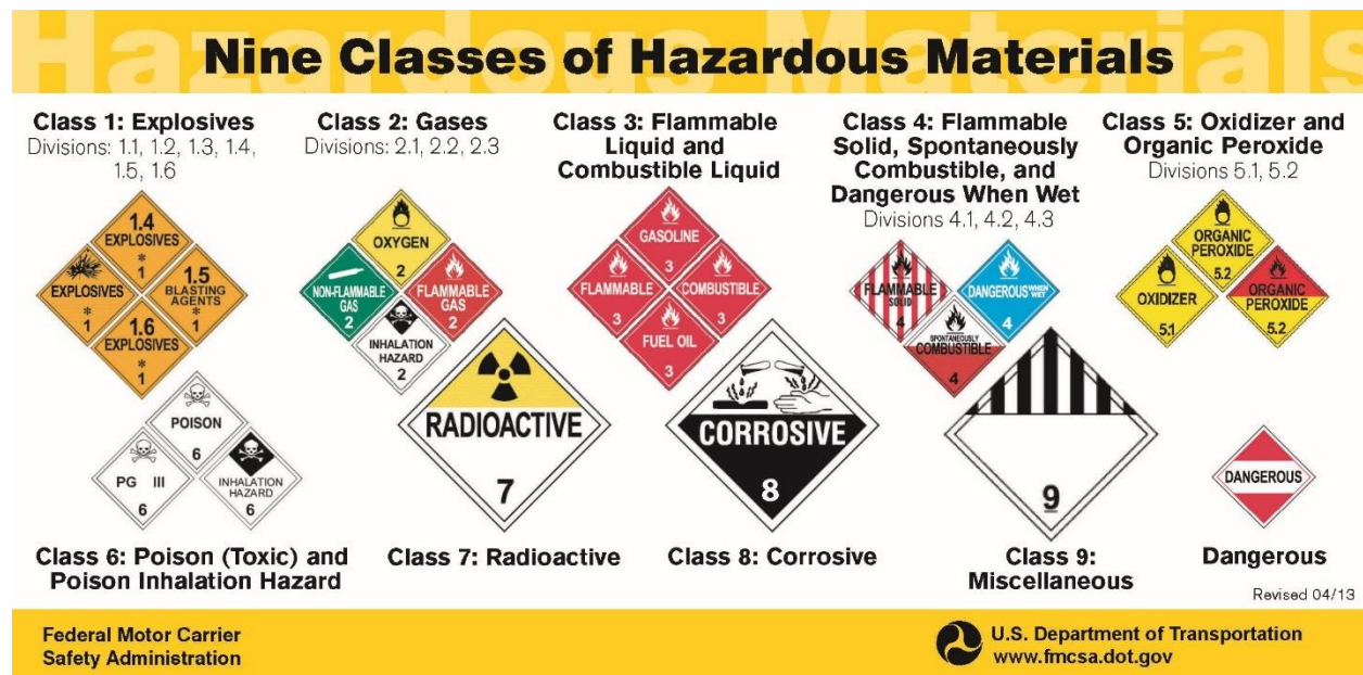
Figure B.29 – Hazardous Materials Classes
