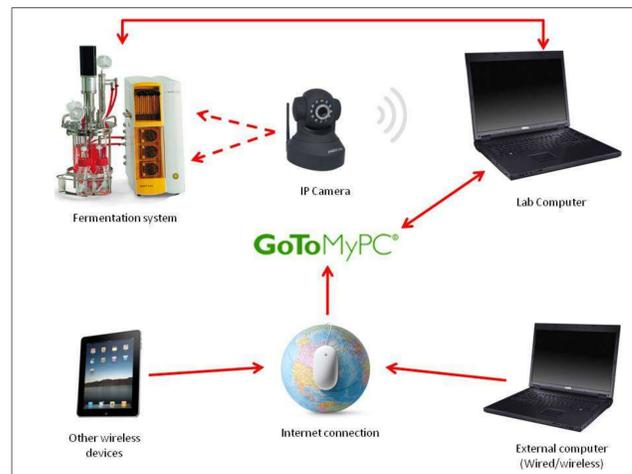
Diagram 1. Networking of the Sartorius-stedim Biostat<sup>®</sup> A Plus fermentation system
